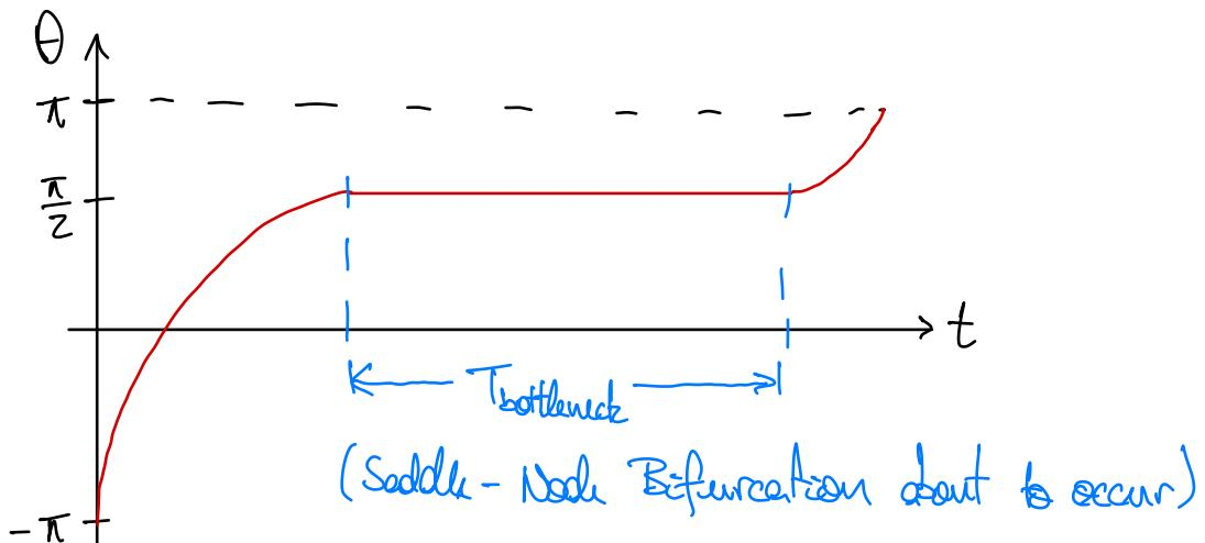
$$\alpha \approx \omega \Rightarrow T = \frac{2\pi}{\sqrt{\omega^2 - \alpha^2}} = \frac{2\pi}{\sqrt{(\omega-\alpha)(\omega+\alpha)}}$$
